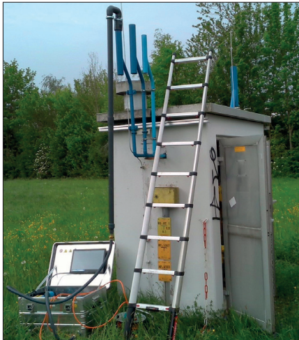
Measurement setup blower (left) and probe array for measuring the leak location on an underground gas pipeline “test section” (right)
