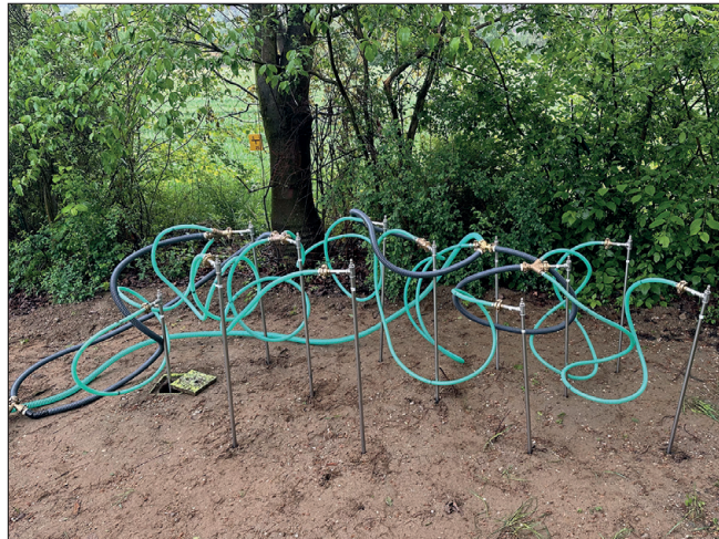
Measurement setup blower (left) and probe array for measuring the leak location on an underground gas pipeline “test section” (right)
